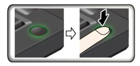
When the fingerprint reader indicator is solid green, tap your finer on the fingerprint reader for authentication.
