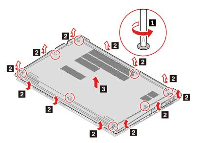
5. Install the new base cover assembly in place 1. Ensure that the latches of the base cover assembly are secured under the base cover assembly 2. Then, tighten the screws to secure the base cover assembly 1.
