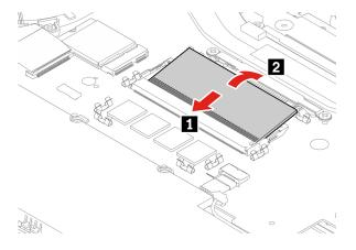
8. Install the memory module bracket as shown 2.
