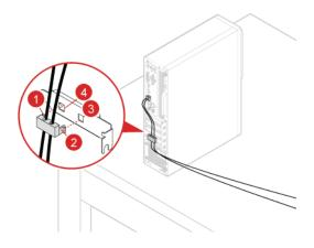
A cable lock can be used to secure devices, such as the keyboard and the mouse, by locking the device cables to the computer. The cable lock connects to the cable-lock slots on the rear of the computer.
