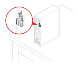
Locking the computer cover helps prevent unauthorized access to the inside of your computer. Your computer features a padlock loop so that the computer cover cannot be removed when a padlock is installed.
