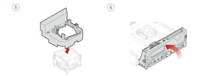
A Reinstall the removed parts. To complete the replacement, see Completing the parts replacement.
