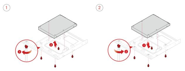
Reinstall the storage converter with the 2.5-inch primary storage drive. See Replacing the 3.5-inch primary storage drive.
