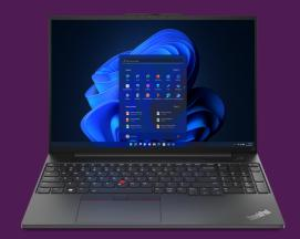
The 16" screen has an optional multi-touch functionality that lets users naturally interact with the device and an anti-glare surface that makes it easier to comfortably work in bright-light conditions. The 16:10 aspect ratio and 100% sRGB color gamut present stunning and true-to-life visuals.
